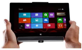
Figure 2: TheEyeTribe Remote Eye Tracker on a tablet
